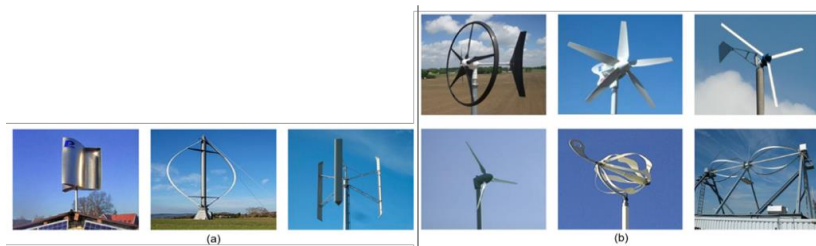
Fig 2. SWTs classification according the axis orientation (a) VAWT and (b) HVWT [38].
