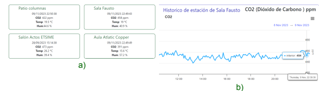
Fig. 3. Visualization of IoT node data in real time (a) summary and (b) full graphic.
