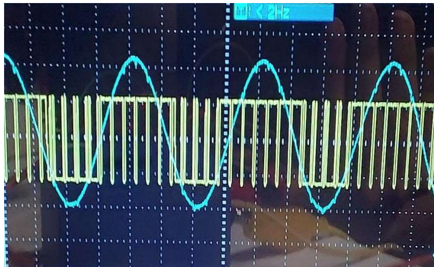
Fig. 5. The carrier signal is shown together with the pulse train generated from it.
