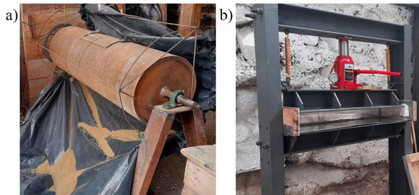
Fig. 1. Equipment for the manufacture of compressed earth blocks. a) Sifting cylinder; and b) Hydraulic press.
